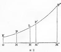
And the main property of the curve is this: that a fourth proportional to any three lines (V being one), OK, MP, M'P', may be found by adding the exponents OM and OM' (making OM"), and finding the line M"P" expounded by that sum. To prove this, make n sets of insertions in OH, and suppose MP to lie between  $V_m$  and  $V_{m+1}$ , while M'P' lies between  $V_{m'}$  and  $V_{m'+1}$ . Now, in the series of continued proportionals,
